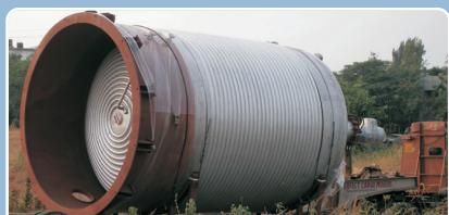
Batch Reactor with Internal and External Coils and Agitator
