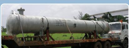
Shell and Tube Heat Exchanger for Oil&Gas
